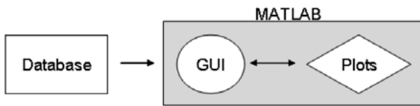
Figure 1. Workflow diagram. MATLAB reads in the database, and the user interacts with the GUI to generate plots until the desired figure is produced.
